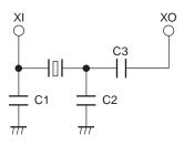
C1 : Used to prevent oscillation at upper harmonic frequencies.
